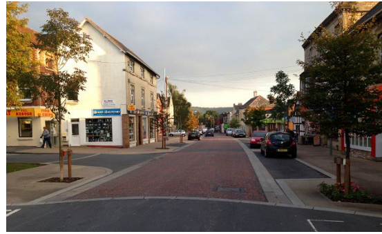
Figure 10 Road Surface Coloring to Reduce Linearity
