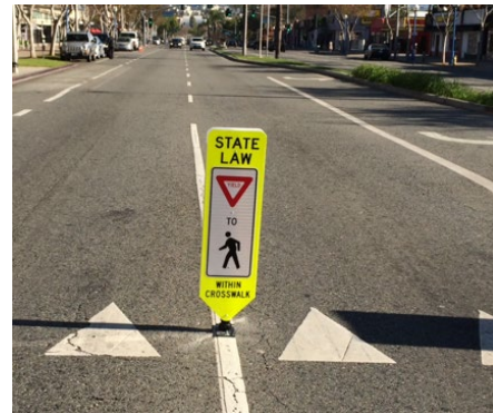
Figure 7 "Pedestrian crosswalk signs" likely have much higher effect on influencing driver behavior not because of the words on the sign, but because their placement in the roadway leads drivers to feel they may collide with the sign.
