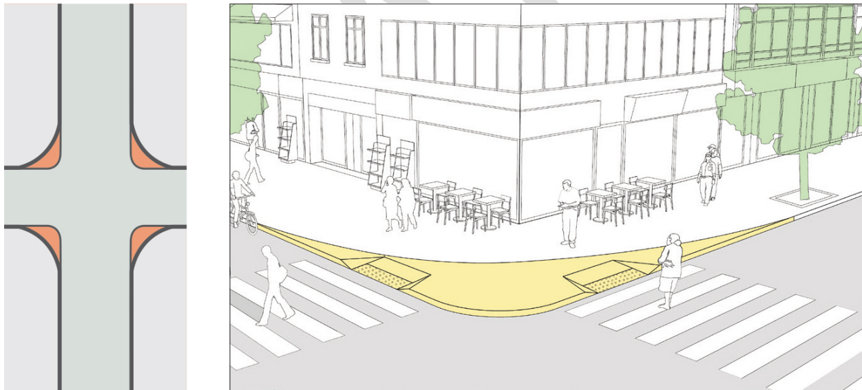
Figure 14 Reducing Corner Radii ( Marked in Red and Yellow) (National Association of City Transportation Officials 2013)
