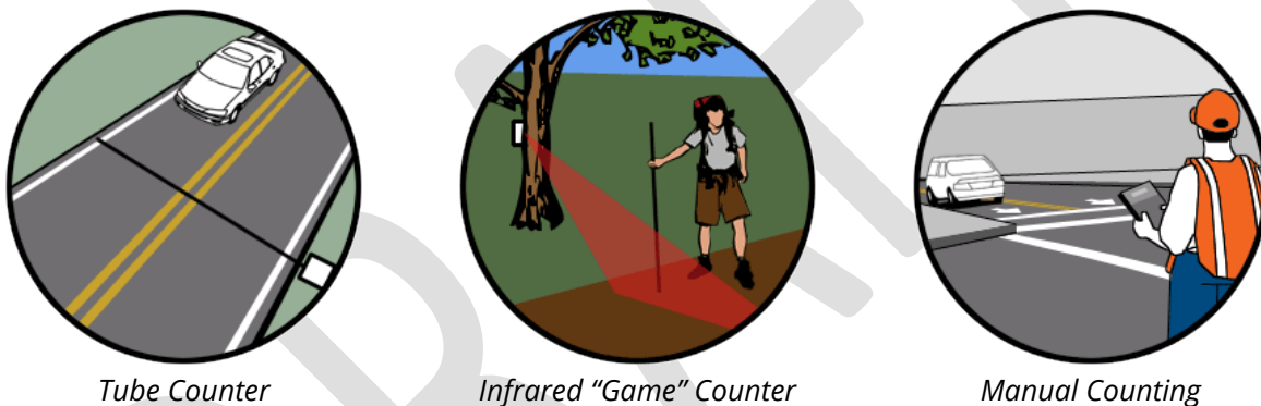
Figure 3 Traffic Counting Methods (Diamond Traffic Products 2019)
