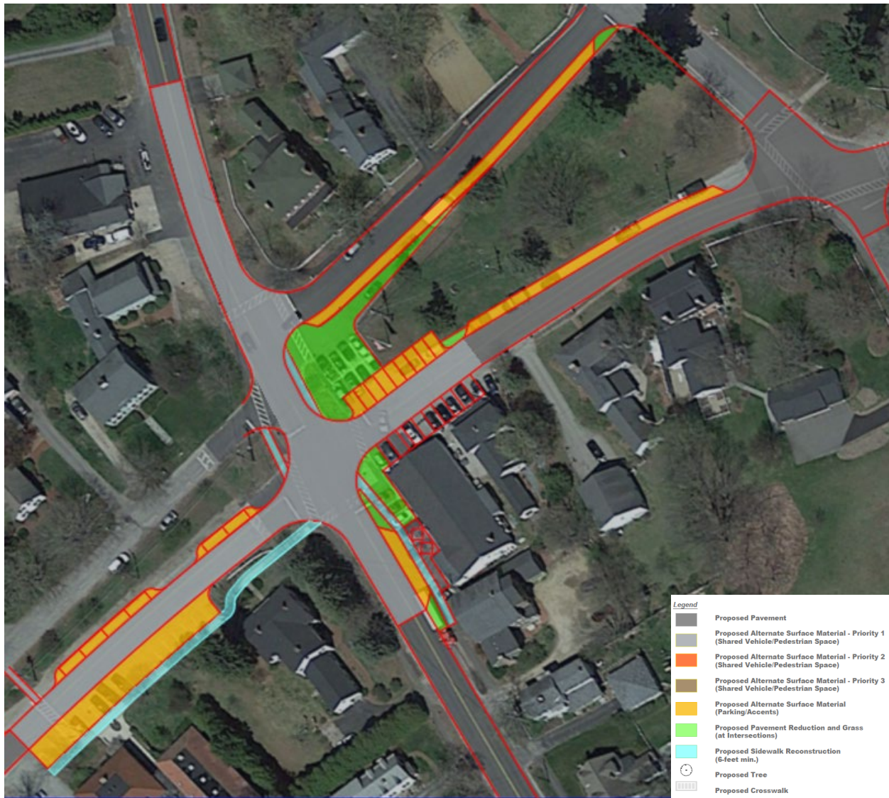
Figure 10. A depiction of recommended improvements for the Carriage Road-Boston Post Road-Main Street-School Street intersection
