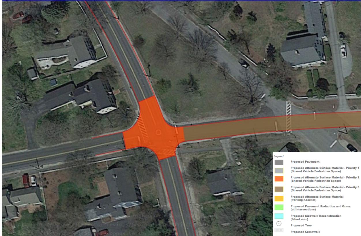
Figure 9. A depiction of recommended improvements for the Boston Post Road-Church Street-Foundry Street intersection
